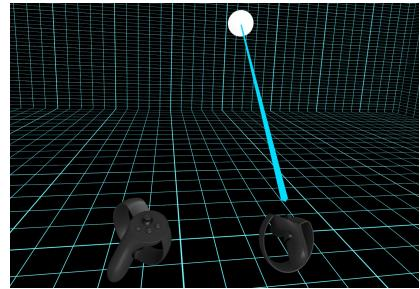
**Figure 1:** Screenshot of the HMD view, which displays both controllers. At the right controller a laser beam with the attached marker approaches. Furthermore, the dark shoebox environment with the rectangular grid is illustrated.
