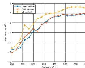
Figure 2: The reproduction relative error comparison of LS, Lasso and OMP method from 250Hz to 590Hz. The reproduction using these three methods are conducted under the same loudspeaker energy constrain.
