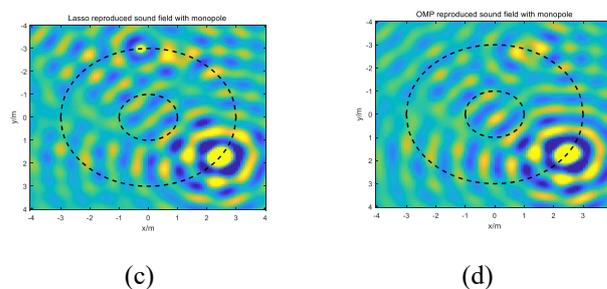
Figure 1: The real part of (a) the target sound field. (b) the field reproduced by LS method. (c) the field reproduced by Lasso method. (d) the field reproduced by OMP method.
