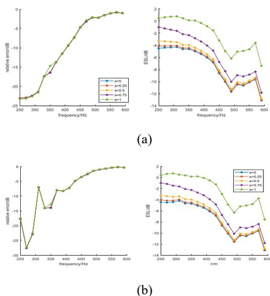
**Figure 4:** Reproduction relative error in the reproduction area and external sound level at the spherical surface  $r=3.2\text{m}$  for (a) the Lasso method (b) the LS method.
