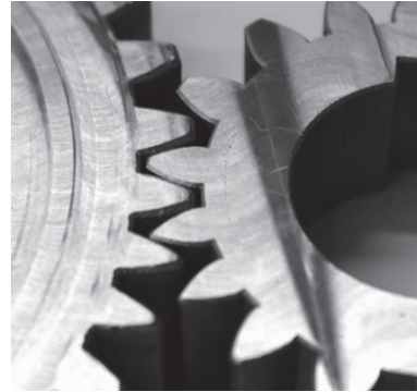
Figure 1: set of inequidistant spur gears with uneven tooth thicknesses and uneven tooth positions
