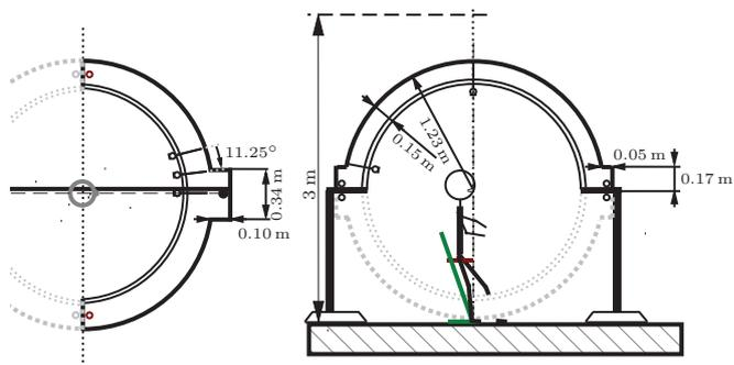
**Figure 1:** Double Circle Microphone Array. Schematic of the measurement setup with two wooden circular rings.
