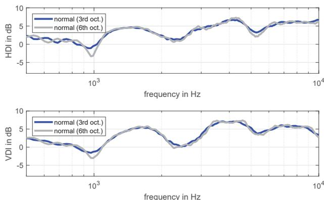
**Figure 3:** Comparison of HDI/VDI values for the glissando method with third-octave and sixth-octave band smoothing (light gray) for "normal" condition.
