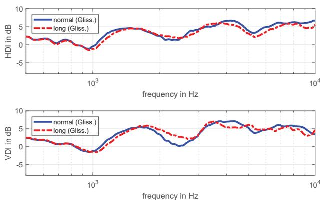
**Figure 6:** Comparison of HDI/VDI values for two mouth openings for the vowel /a/ with the glissando method.
