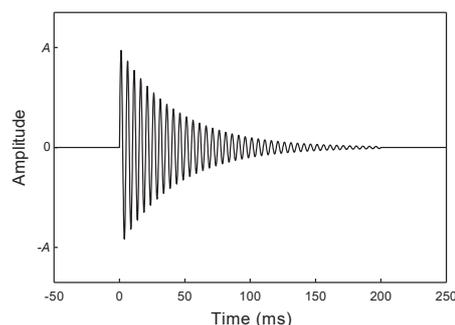
**Figure 2:** A base waveform of feedback stimuli that emulates the natural response of touch buttons. The frequency and amplitude were determined by considering the threshold level of the human tactile and auditory senses. Twelve tactile feedback stimuli and eight auditory feedback stimuli were created for the psychophysical experiment.
