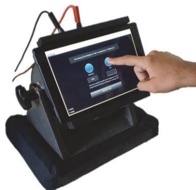
**Figure 1:** An experimental apparatus that consists of a touchscreen tablet and an electric dynamic shaker. A graphical user interface was designed by MATLAB and was displayed on the screen for the evaluation task.
