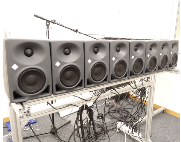
Fig. 1: Example prototype using 8 Neumann KH 80 DSP loudspeakers with a spacing of 154 mm
