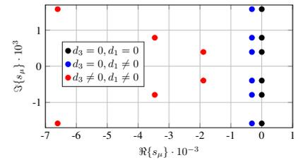
**Figure 3:** Pole-zero plot of the plate for three different damping scenarios.
