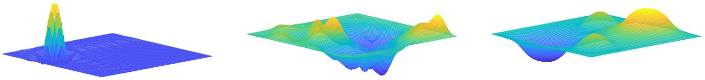
**Figure 4:** Spatial distribution of the deflection  $w(x, y, t)$  at  $t = 0$  while the excitation by a single impulse (left),  $t = 0.1\text{s}$  shortly after the excitation (mid) and in the release phase  $t = 0.6\text{s}$  (right)
