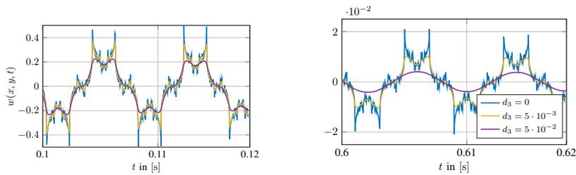
**Figure 2:** Temporal progression of the deflection  $w(\mathbf{x}, t)$  on the plate for different frequency dependent damping ( $d_3$ ) shortly after the excitation (left) and in the release phase (right)
