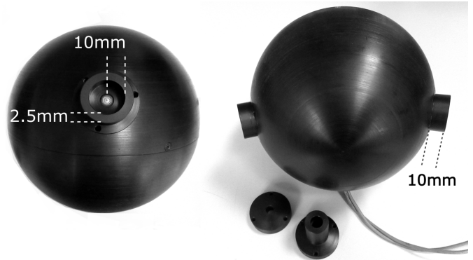
Figure 1: Side and top view of the resonator sphere . KE4 microphones are inserted through a bottom opening of the PVC sphere, and fastened to the bases of the small cylinders.
