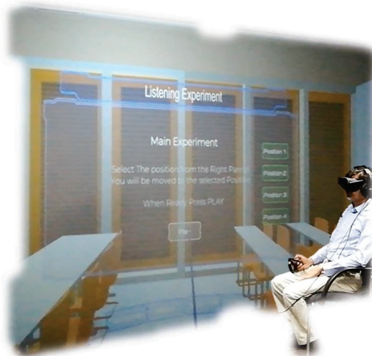
Figure 1: Virtual reality building acoustics auralization environment listening experiment setup [9]
