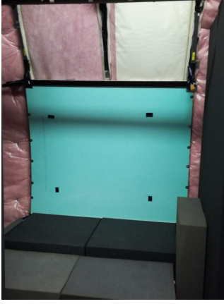
Figure 6: Installed sidewall panel inside the acoustic flight lab demonstrator for Transmission loss type (i.e. noise reduction) test under random acoustic loads.
