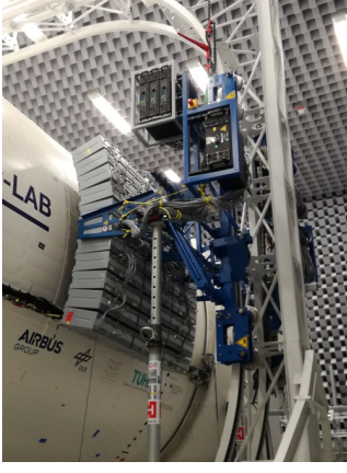
Figure 5: Location of array of loudspeakers on fuselage used for random acoustic excitation on external fuselage skin
