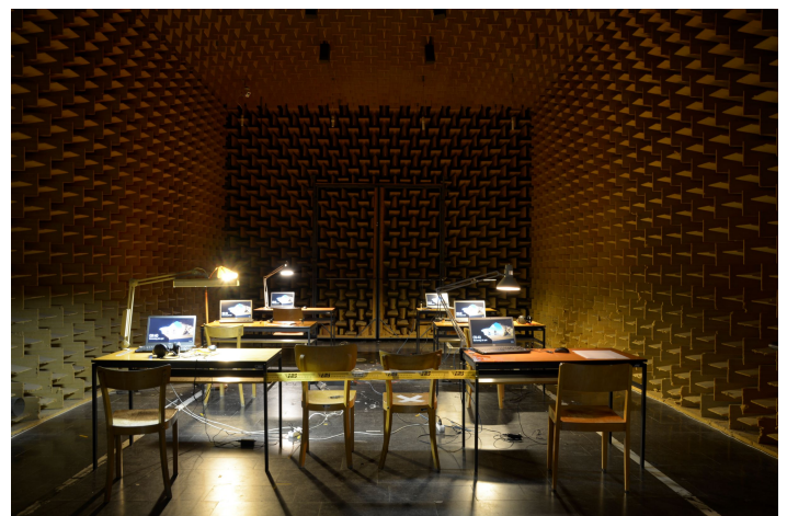
Figure 3: Setup of the listening test. The test was conducted in the hemi-anechoic chamber, providing a larger space than a hearing booth and low environmental noise. Additionally, spotlights at the desk should further fade out the environment and its geometries.
