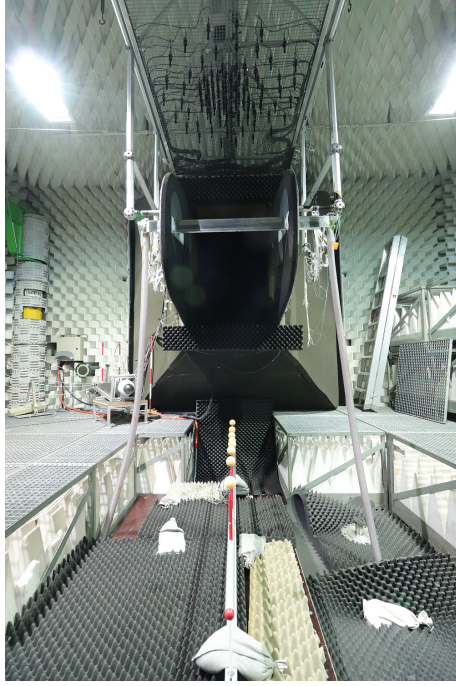
Figure 3: Experimental setup in the AWB. Phased microphone array above the test section. Free-field microphones below the test section.
