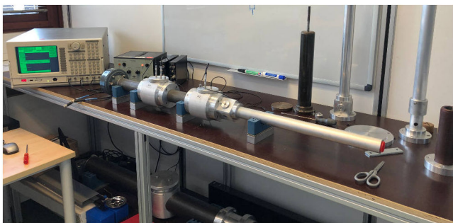
Figure 3: Transmission tube with internal diameter of 45mm with two measurement heads and closing impedance. Total length is 1.4 m
