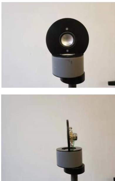
Figure 1: Manufactured variable-directivity loudspeaker, the upper is the dipole part and the lower is monopole part.
