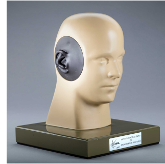
Figure 1: Type 3.3 ear simulators mounted on dummy head Harry. The ear simulators can be replaced by Type 3.4 simulators.
