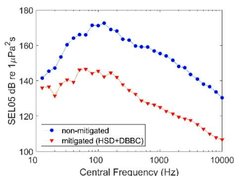
**Figure 4:** Example of an analysis with MarinEARS: comparison of the SEL<sub>05</sub> measured for pile driving events in the German EEZ with and without the application of technical sound abatement systems.
