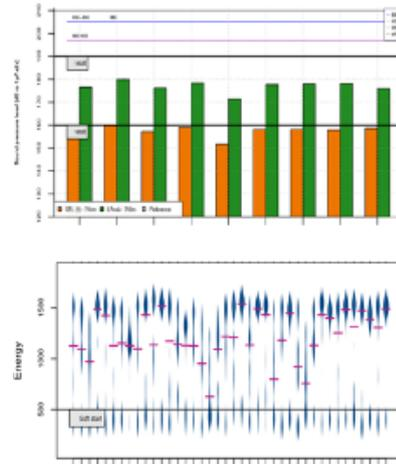
**Figure 2:** Top: Sequence of SEL<sub>05</sub> and L<sub>p,pk</sub> for different piles of a wind farm: The threshold values at activity level were met. Bottom: Distribution of hammer energy applied during pile driving for different piles of an offshore wind farm.
