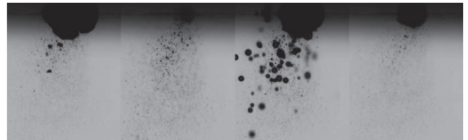
Figure 3: Large, medium and small bubbles for low amplitude pressure field. The gray horizon on the top is the sonotrode tip surface. Time difference between each image is 66.6 \mu\text{s} , and the frame width is 1.13 mm.
