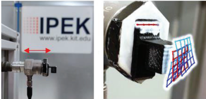
Figure 3: ABSplus resonator mounted on the impedance sensor with measurement points in min, zero and max position (right) [1]
