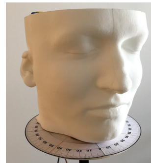
Figure 2: 3D printed head model used for freefield and room measurements. Two electret microphones have been inserted at the entrance of the left and right ear canal. The head is life-sized and modelled after a CT-scan. Dimensions are 20 cm x 18 cm x 16 cm (length x width x height). Fabricated at the Institute of Micro Technology and Medical Device Technology, Technical University of Munich.
