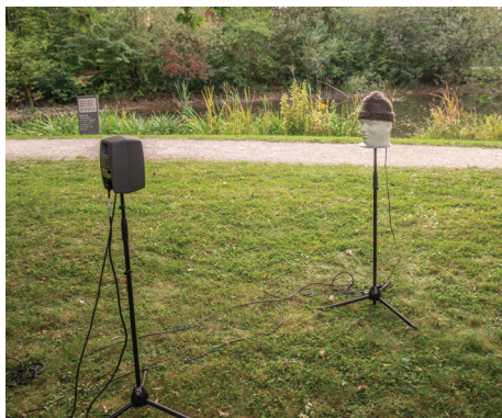
Figure 3: Measurement setup in freefield conditions to reduce impact of reflections on model output. Speaker was oriented towards open space (lake) with a distance of 150 cm to the physical head model.
