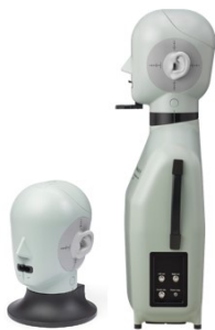
Figure 13: A realization of the ear simulator in a HATS is commercially available. The two HATS configurations are named Type 5128-B-111 and Type 5128-C-111.
