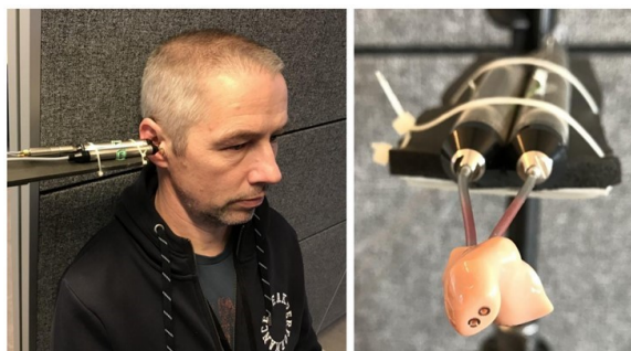
Figure 9: The photo shows a person where the microphone arrangement has been attached to the individual earplug. The individual earplug attached to the microphone arrangement and at the end of the earplug the two tubes can be observed.
