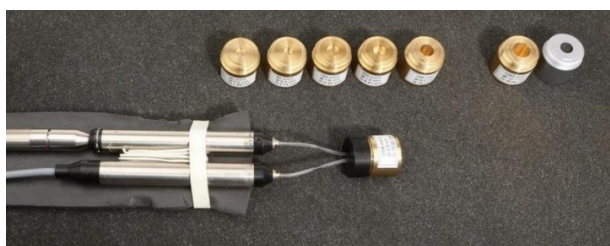
Figure 8: The photo shows the microphone arrangement used for the measurements as well as the reference volumes required for the calibration of the microphone arrangement. In the photo one of the reference volumes are connected to the microphone arrangement via two soft flexible tubes.
