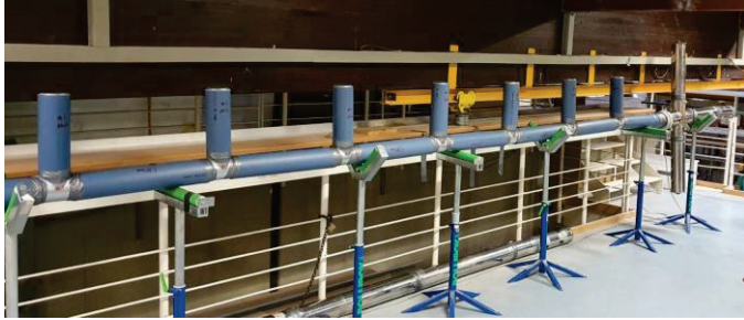
Figure 11: Test setup with seven quarter-wave resonator.
