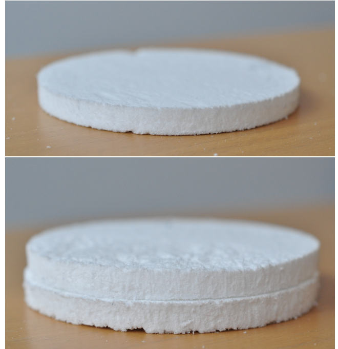
Figure 1: Two flexible aerogels based on methyltrimethoxysilane and dimethyldiethoxysilane. Top: material “ Basic ” with a density of 110 \text{ kg/m}^3 and a thickness of 9 mm. Bottom: material “ Diluted ” with a density of 70 \text{ kg/m}^3 and a thickness of 18 mm.
