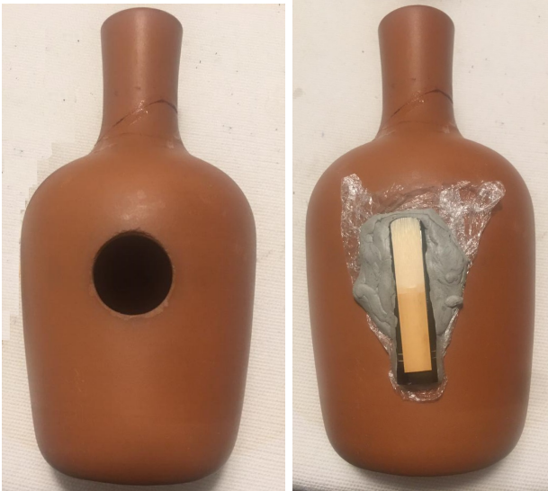
Figure 1: The Brazilian moringa (left) with a truncated clarinet mouthpiece and reed (right). In all excitation methods the reeds and mouth were adapted to the lateral hole
