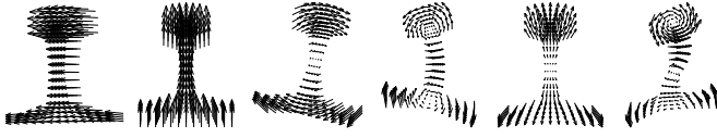
Figure 4: Some wave types as calculated by the WFEM. From left to right: lateral bending, vertical bending, torsion, web bending (second order torsion), expansion, third-order torsion.
