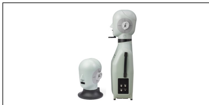
Figure 14: A commercially available physical realization of the Type 4.3 Ear Simulator according to ITU-T P.57.
