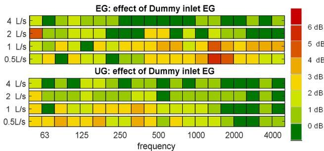
**Figure 5:** The difference between the averaged blocked force of the straight pipe (#2) and that of the straight pipe with the tee on the ground floor (#3), measured on the ground (top plot) and on the underground floors (bottom plot) at different volume flow rates.
