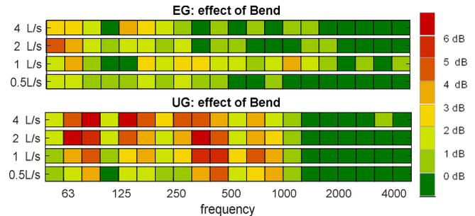
**Figure 4:** The difference between the averaged blocked force of the straight pipe (#2) and that of the straight pipe with the basement bend (#5), measured on the ground (top plot) and on the underground floors (bottom plot) at different volume flow rates.
