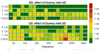
**Figure 6:** The difference between the averaged blocked force of the straight pipe (#2) and that of the straight pipe with the tee on the underground (#4), measured on the ground (top plot) and on the underground floors (bottom plot) at different volume flow rates.
