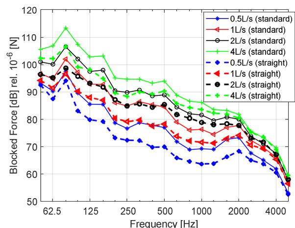
**Figure 3:** The averaged blocked force of the standard pipe (#1, solid lines) and the straight pipe (#2, dashed lines) measured on the underground floor with the volume flow rates of 0.5 L/s (blue), 1.0 L/s (red), 2.0 L/s (black), and 4 L/s (green).
