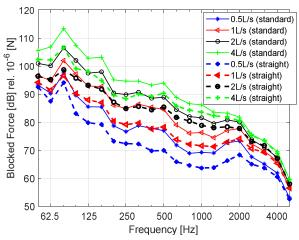
**Figure 3:** The averaged blocked force of the standard pipe (#1, solid lines) and the straight pipe (#2, dashed lines) measured on the underground floor with the volume flow rates of 0.5 L/s (blue), 1.0 L/s (red), 2.0 L/s (black), and 4 L/s (green).
