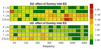
**Figure 5:** The difference between the averaged blocked force of the straight pipe (#2) and that of the straight pipe with the tee on the ground floor (#3), measured on the ground (top plot) and on the underground floors (bottom plot) at different volume flow rates.
