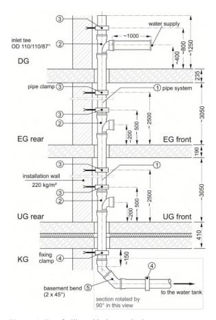
**Figure 1:** Test facility with the standard wastewater system set-up at IBP, Stuttgart for measurements according to DIN EN 14366 [1].
