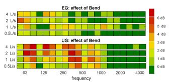
**Figure 4:** The difference between the averaged blocked force of the straight pipe (#2) and that of the straight pipe with the basement bend (#5), measured on the ground (top plot) and on the underground floors (bottom plot) at different volume flow rates.
