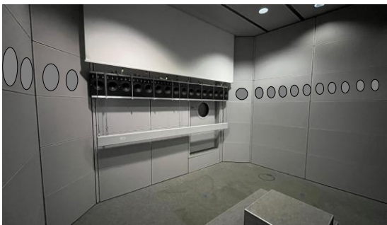
Figure 2: WFS system at the TU Dresden
