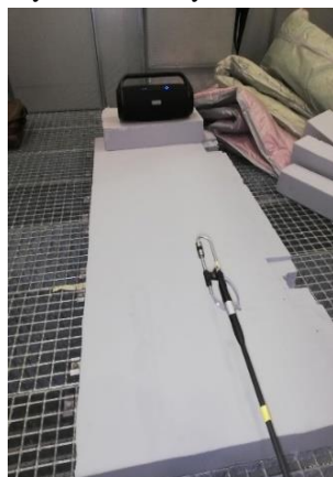
Figure 13 : Sound intensity measured without box in free field room of FTZ -Akustik laboratory.
