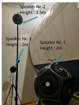
Figure 3 :Excitation in acoustic chamber with three loud speaker.
