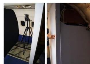
Figure 6 : Sound pressure measurement in Bear cave on panel without carpet.
