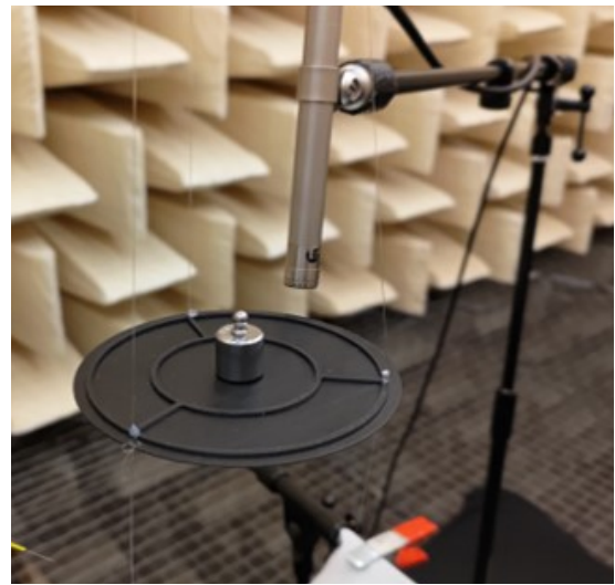
(a) The 'hanging plate' design with an effective diaphragm area of 82.3 cm 2 .
