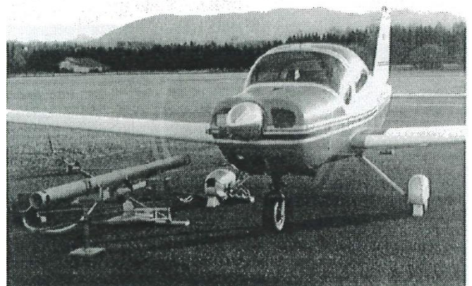
Figure 1: flyable ANC system for a Bölkow Monsun Bo 209 using a linear arrangement of four anti-sound actuators in a tube-like structure [8]
