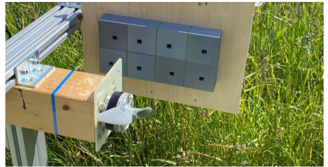
Figure 3: propeller/AMM mockup for acoustic measurements
