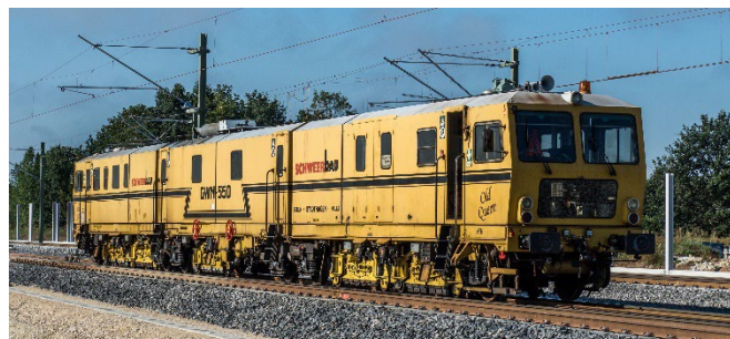
Figure 1: Grinding vehicle GWM 550, Photo: customized (tailored) ‘Schweerbau-GWM-550-Schienenschleifmaschine’, Reinhold Möller, https://commons.wikimedia.org/wiki/File:Schweerbau-GWM-550-Schienenschleifmaschine-P8115004.jpg , CC BY-SA 4.0.
