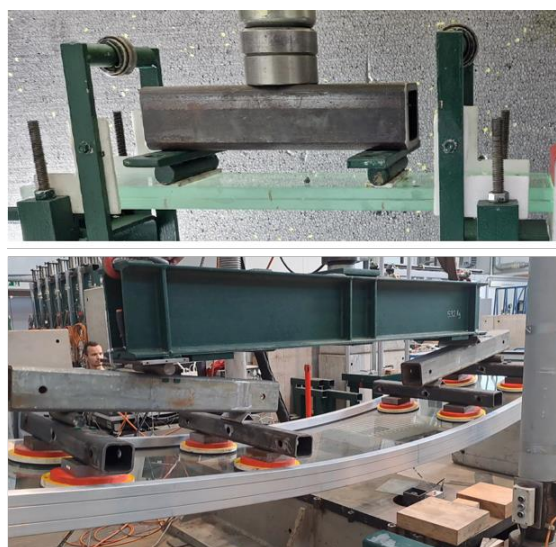
Figure 3: Testing the bending load capacity of a small LSG sample (top) and the full-scale noise-reducing element (bottom) (photos: MFPA Leipzig).
