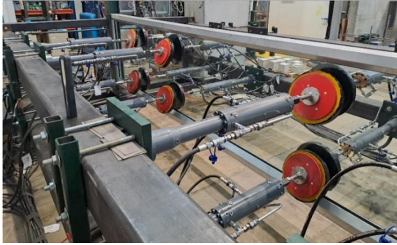
Figure 4: Testing fatigue strength of a small LSG sample (top) and the full-scale noise-reducing element (bottom) (photos: MFPA Leipzig).
