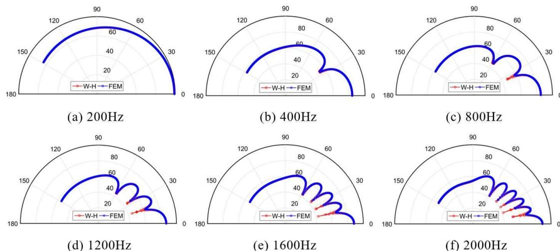
Figure 5 – Directivity patterns of the radiated sound fields (Sound pressure level/dB) obtained by the Wiener-Hopf technique and the FEM at different frequencies ( $r=5m$ )
