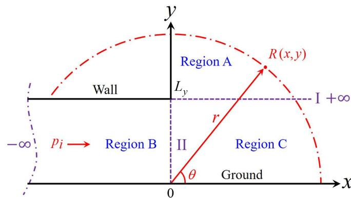
Figure 1 – Schematic diagram of sound radiation from un baffled long enclosure with ground
