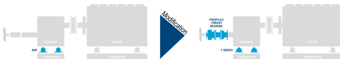
Figure 7 – Drivetrain modification case 2: Replacing semi-elastic gearbox mounts by a soft gearbox mounting systems in combination with a propeller shaft coupling and an additional thrust bearing.
