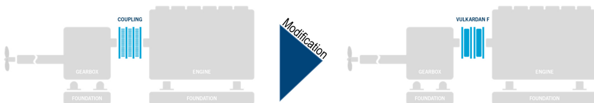
Figure 5 – Drivetrain modification case 1: Installing a two-row coupling with low torsional stiffness and additive intermediate mass
