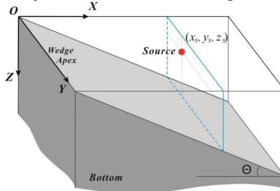
Figure 4 – Geometry of a wedge-like waveguide
