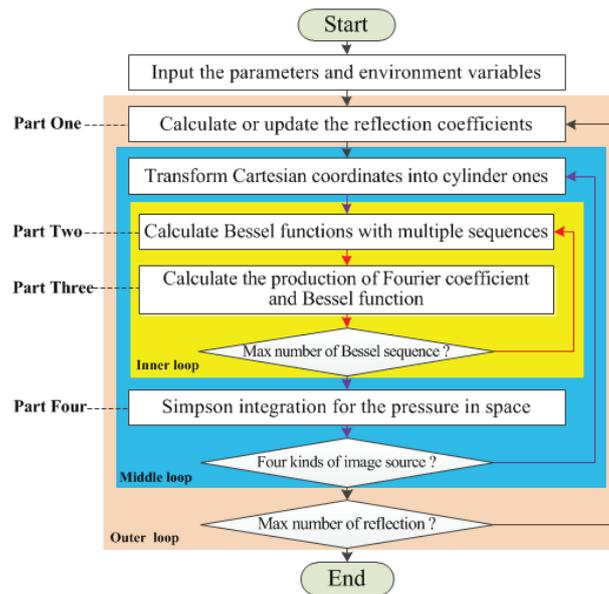
Figure 6 – Computational flow of the acoustic field by image source method
