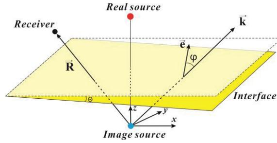
Figure 3 – Image source for inclined interface
