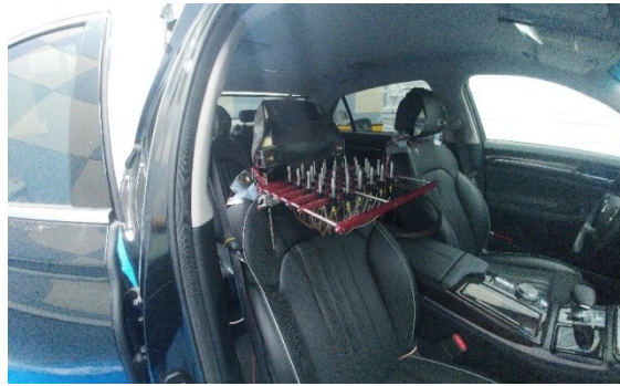
Figure 1. Measurement with a planar array of microphones in a car cabin (by courtesy of Jung-Woo Choi)
