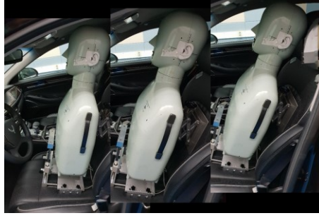
Figure 2. Positioning of the dummy head microphone (leaning 1/2/3)
