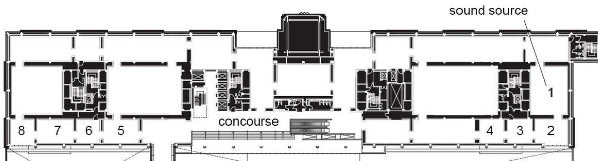
Figure 1 – Floor plan of two sequential spaces, concourse and the location of sound source
