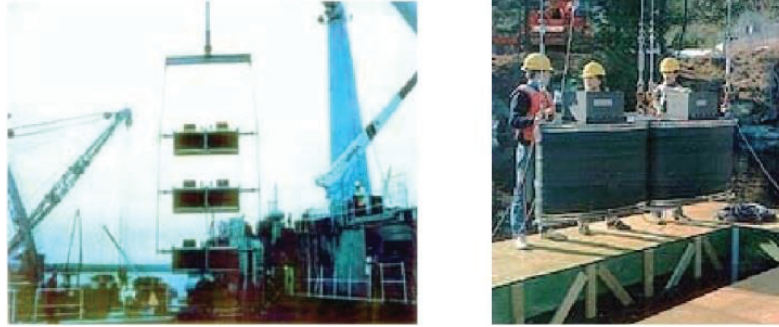
Figure 6-Towed low-frequency active sonar (SURTASS-LFA)
