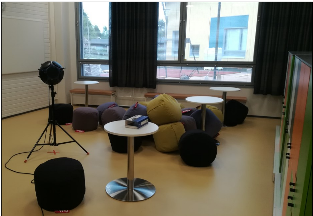
Figure 3 – An example of the measurement setup in an open plan school. The microphone positions are to be on a straight line from the speaker to the right behind the cabinets.
