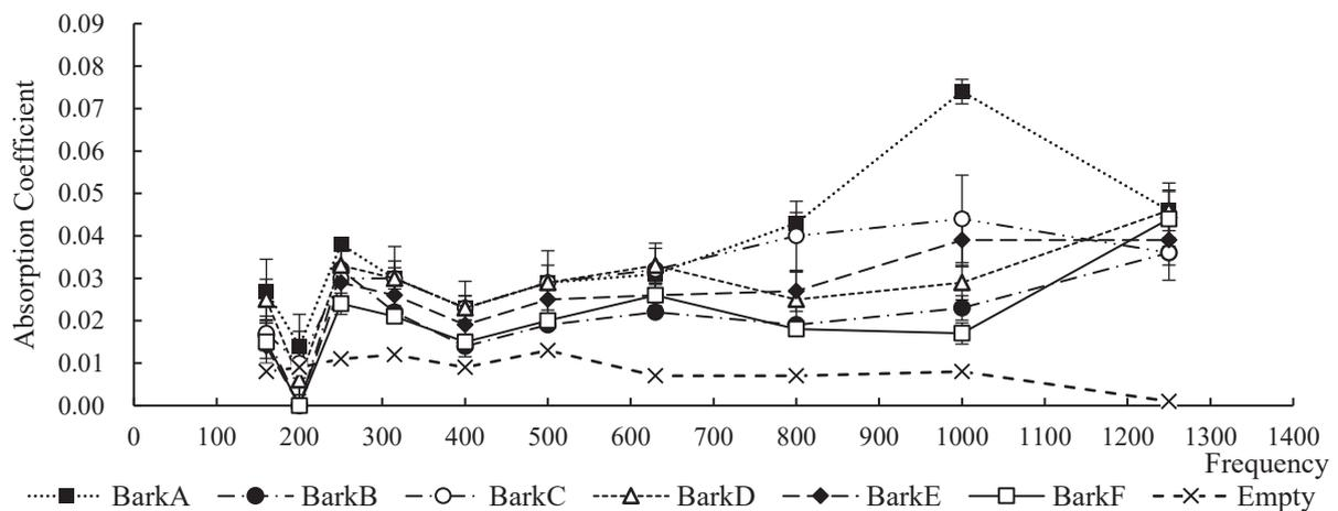
Fig.2 Absorption Coefficient for 6 plants
