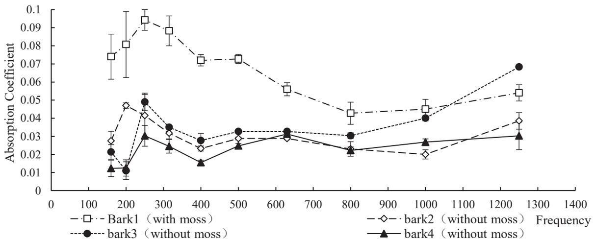
Fig. 5 The difference of absorption between bark with moss and without moss
