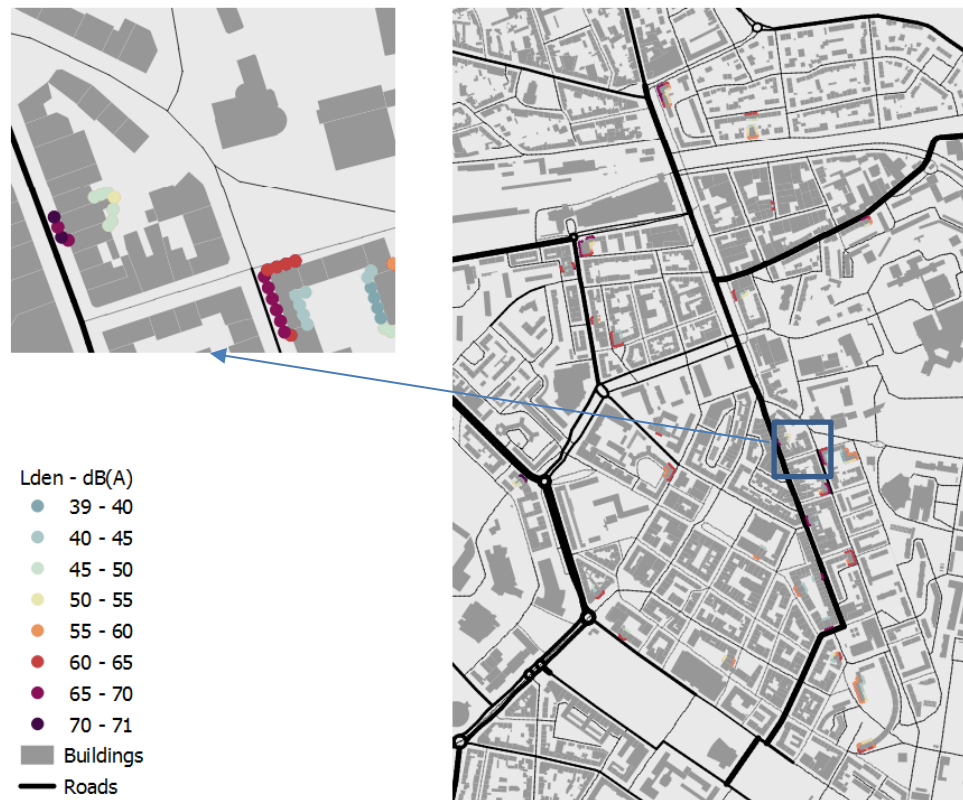
Figure 2 – Noise map of the study area computed with NoiseModelling (median sound level of the 100 simulations). Following this map, the inhabitants ratio exposed to L_{den} > 65 dB(A) is about 17 %.
