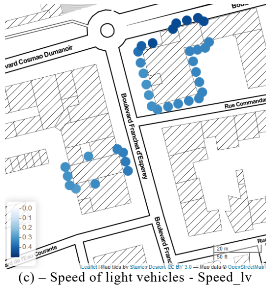
Figure 4 – L_{den} variation ( \mu^* ) by receiver of the sensitivity analysis for 3 input parameters
