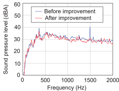
Figure 11 – Comparison of frequency characteristics between original sound and after improvement
