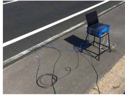
Figure 6 – (left) Procedure for the determination of the mechanical impedance (14) – (right) Actual setup
