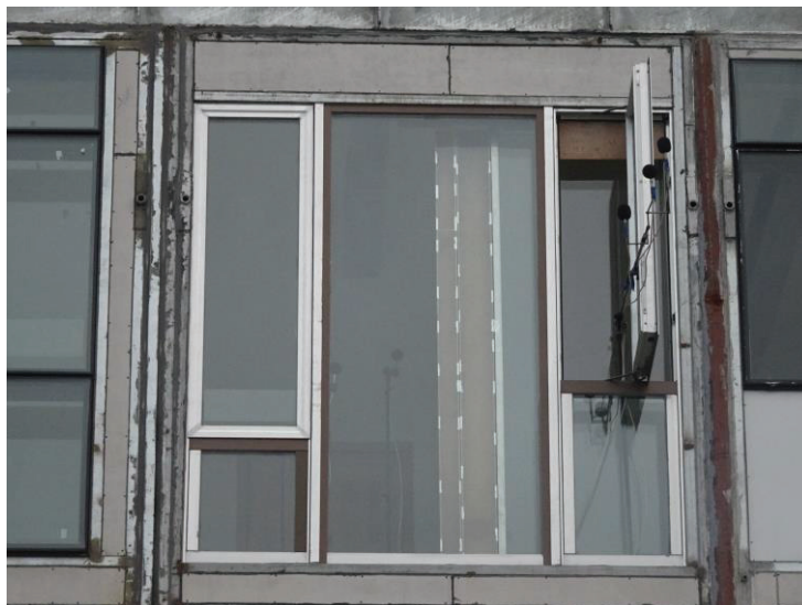
Figure 2 Window 1 tested with increasing overlapping. The view from outside shows the outdoor microphone location and the largest overlapping length
