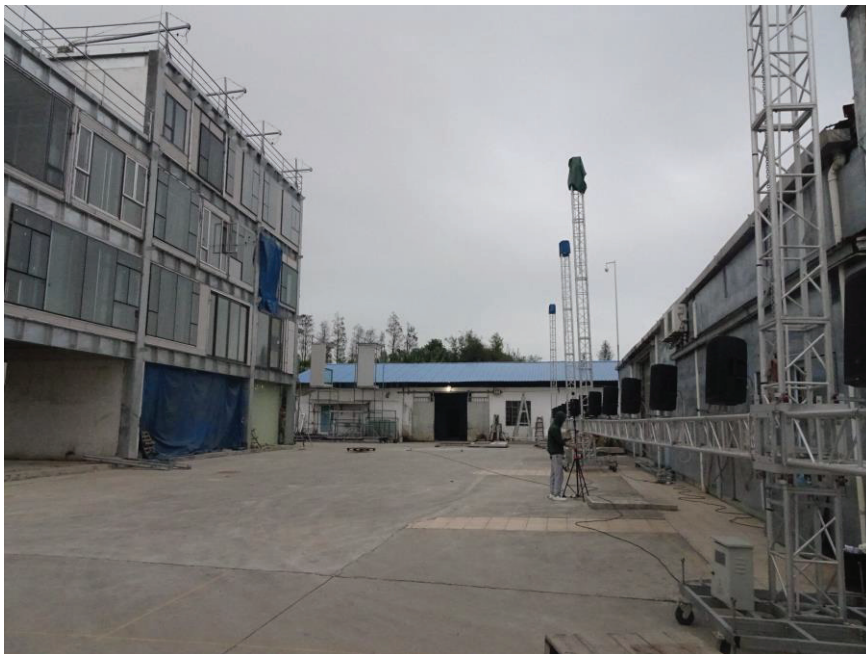
Figure 1 Set up of the Off-site mockup test. The array of loudspeakers is placed parallel to the testing façade, which create a 0° line source angles
