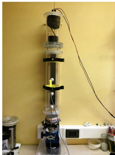
Figure 2. Experimental setup for measuring the normal-incidence sound absorption coefficient of the membrane absorber
