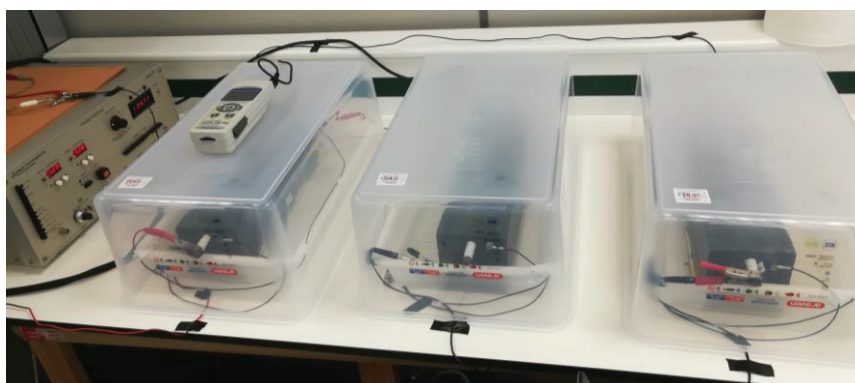
Figure 3 – Experimental setup of the forced corrosion test
