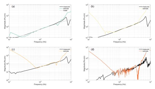
Figure 6. Frequency response function of the specific acoustic impedance (see Eq. Eq. (5)) of (a) the loud-speaker mounted in a baffle in anechoic chamber, (b) the closed-box loudspeaker mounted in a baffle in anechoic chamber, (c) the closed-box loudspeaker placed in an anechoic room and (d) in a lightly damped room.
