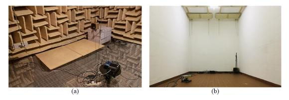
Figure 4. Experimental setup for estimating the front-side acoustic load impedance on the closed-box loud-speaker system (a) placed in an anechoic room and (b) located near a corner in a lightly damped room.
