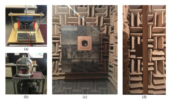
Figure 2. Experimental setup for measurement of the electrical impedance of the loudspeaker driver (a) when the coil is blocked, (b) in vacuum, and (c) mounted in a baffle in open space. In (a), a specific locking system is used to prevent the diaphragm from vibrating, and thus the coil attached thereto; in (b), the loudspeaker driver unit is placed in a vacuum chamber to eliminate the effect of air on the diaphragm; in (c), the loudspeaker driver is mounted in a baffle in an anechoic chamber.
