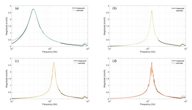
Figure 5. Frequency response function between the input current and the output velocity as given in Eq. (4) of (a) the loudspeaker mounted in a baffle in anechoic chamber, (b) the closed-box loudspeaker mounted in a baffle in anechoic chamber, (c) the closed-box loudspeaker placed in an anechoic room and (d) in a lightly damped room.
