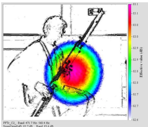
Figure 1: C5 first mode with  $f = 523.3$  Hz
