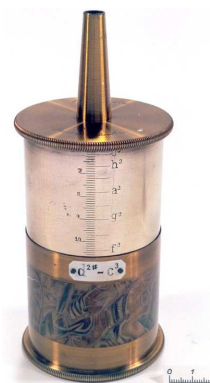
Figure 3: Resonator no. 4 with the length adjusted to l = 107.5 mm.
