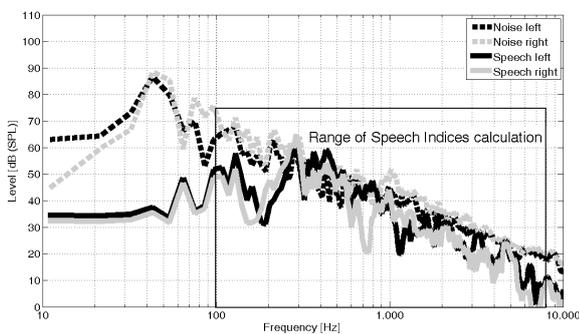
**Figure 1:** Spectra of typical speech and noise in cars.
